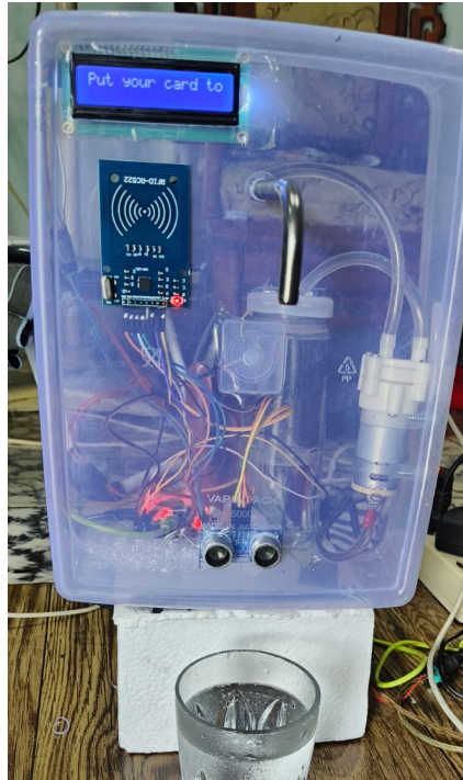
Gambar 7. Prototipe smart water dispenser berbasis Internet of Things
