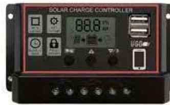
Gambar 5 Solar charger control
