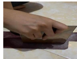
b. The process of sanding the remaining remaining PCB size
