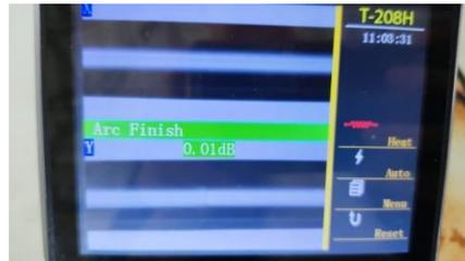
Fig.15 Results of connecting the drop core cable to the first two connection connections
