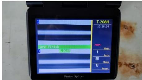
Fig.14 Results of connecting a single connection drop core cable
