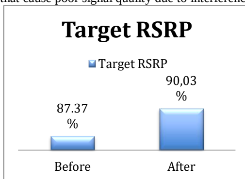
Figure 9. Percentage Grafik image of the result of changing the tilting method of the antenna
