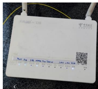
Figure 4. ONT Condition Has Been Activated by FTTH Network
