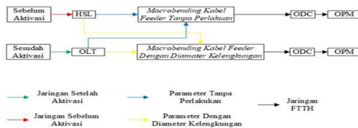
Figure 5. Block diagram of macrobanding in the feeder cable segment
