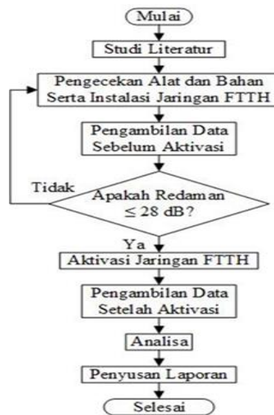
Figure 1. FTTH network installation and activation design flow
