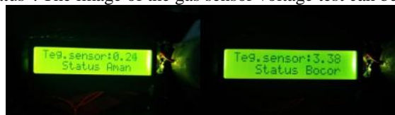
Figure 7. Sensor Testing for Safe and Leaking Conditions
