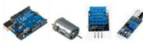
Fig. 2 Components of the automatic sieving tool (a) Arduino Uno (b) DC motor (c) DHT11 (d) IR sensor
