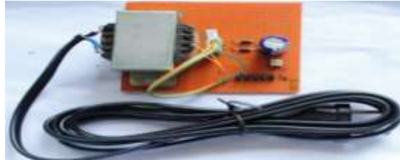
Figure 2. Power Supply Circuit (source: personal documentation)
